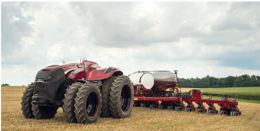
Fig. 1 Autonomous tractor concept – Case IH
